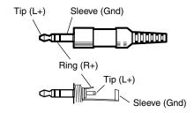
Figure 2-14 — Audio input connector wiring
